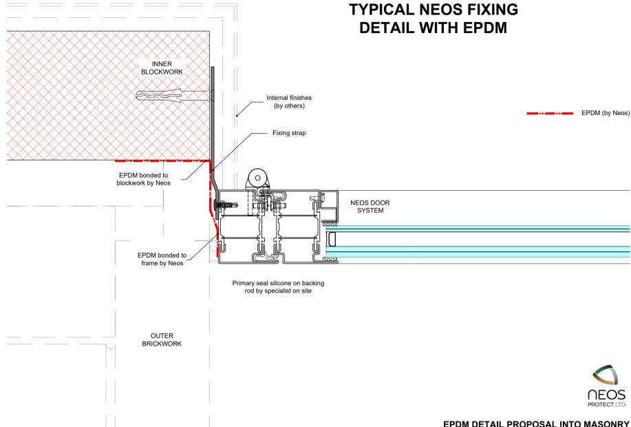
EPDM DETAIL PROPOSAL INTO MASONRY INSTALL PRIOR TO CONSTRUCTION OF OUTER SKIN OF BRICKWORK
