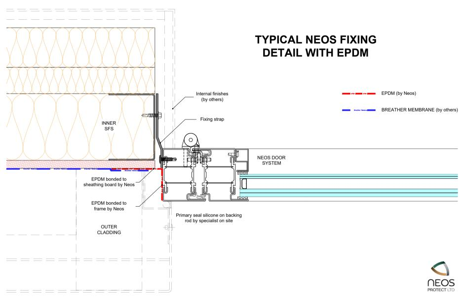
EPDM DETAIL PROPOSAL INTO SFS DOOR / SCREEN INSTALL PRIOR TO INSTALLATION OF OUTER CLADDING
